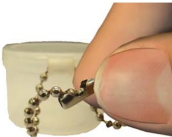
Fig 1. Fixing of Metal Chain
